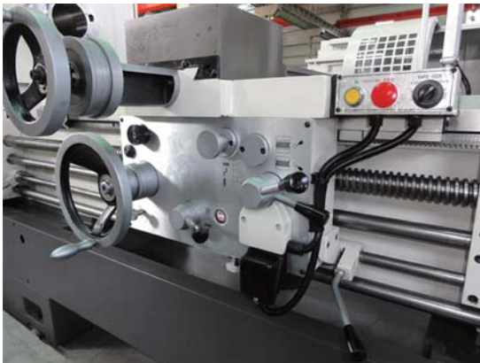
Powerful apron Rapid traverse and controls on carriage 2 clamp down bolts for high rigidity top slide
