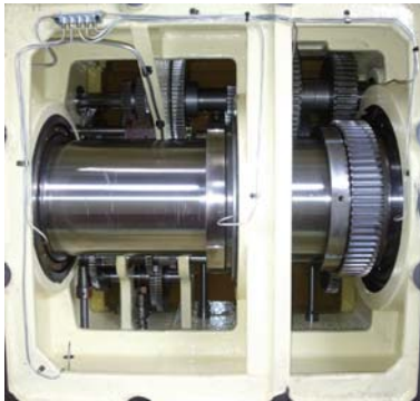
Powerful apron Rapid traverse and controls on carriage 2 clamp down bolts for high rigidity top slide
