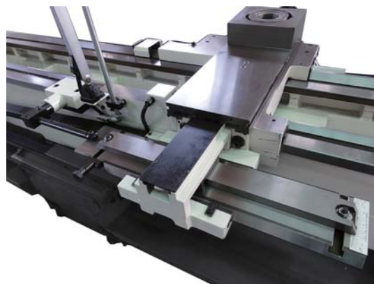
Heavy duty taper attachment
