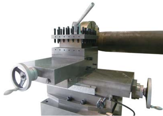
Cross and longitudinal compound rest
